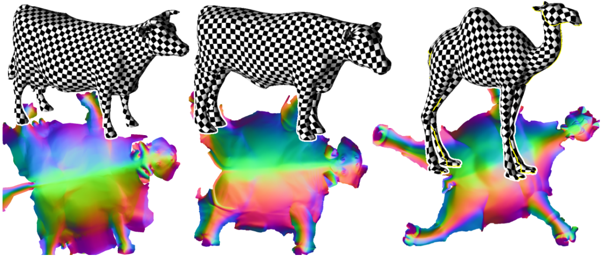
Figure 4.8: Some results computed by stretch L_2 minimization (parameterized models courtesy of Pedro Sander and Alla Sheffer).
